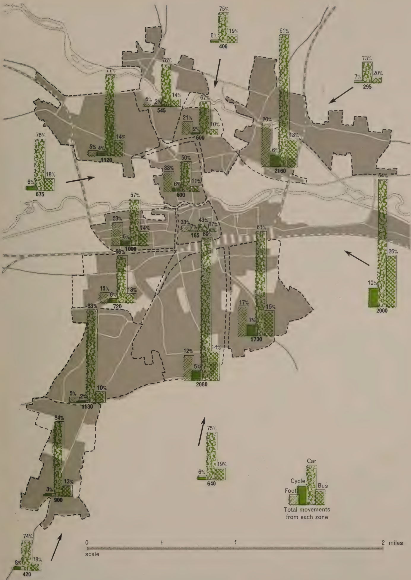
77 Mode of travel for the journey to work from each residential zone in year 2010 including residential zones outside the city (indicated by arrows).
